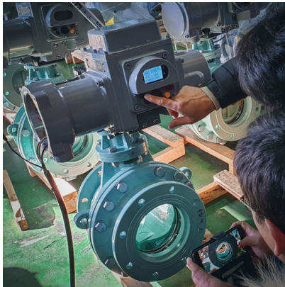
200A Ball Valve (1,100 Nm)
